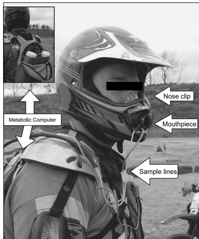
**FIGURE 1**—Ambulatory oxygen consumption measurement while riding an off-road vehicle. The rider's nose is plugged and all expired air is expelled through the mouthpiece which contains a volume meter and expired air sample line held in place by the modified chin guard of the helmet. *Inset top left:* Reverse angle view of the metabolic computer (with protective padding) in the backpack as worn by riders.
